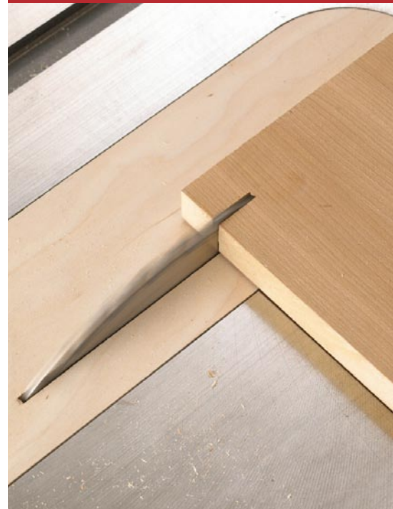
This shop-made zero-clearance insert fully supports delicate veneer fibers as the blade's teeth exit the cut.
